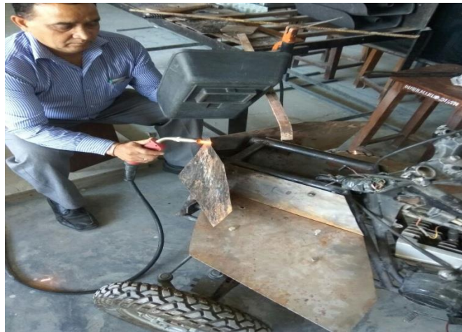
Fig 3: Welding on the chassis and body
