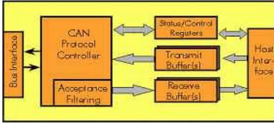
FIG 1. Block Diagram of CAN
