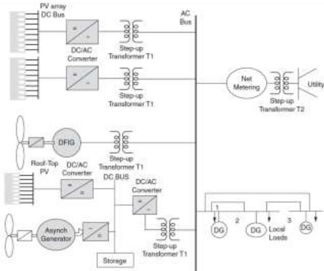
Fig.2 (a) shows AC Microgrid
