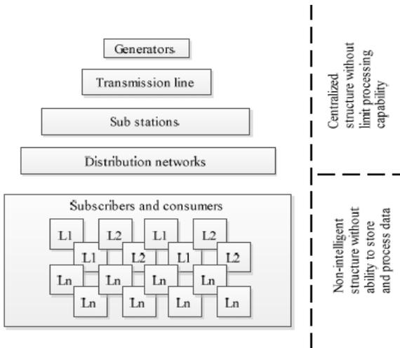
Fig 4(a).Shows Block Diagram of Conventional Grid
