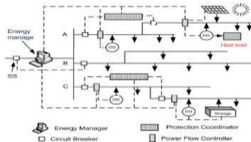
Fig.1.Shows Architecture of Microgrid [7].
