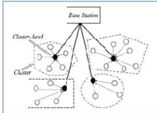
Figure 1. Communication Architecture of protocol LEACH
