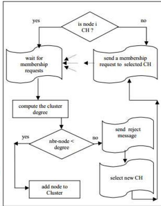
Figure 6. Clustering Stages in WB-TEEN
