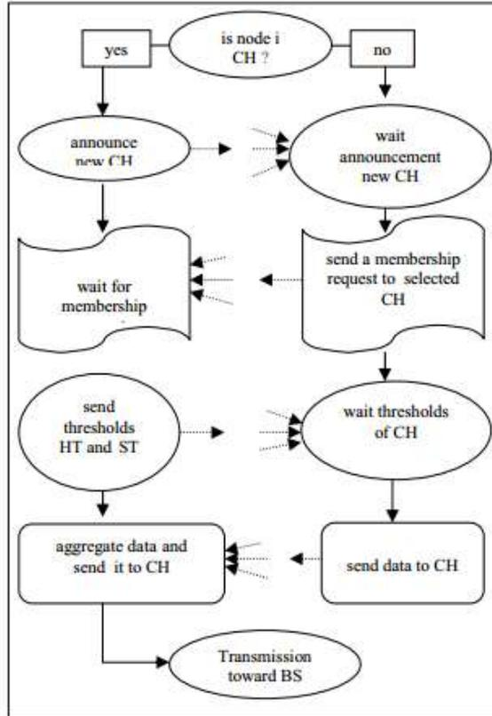
Figure 3. Initialization, Search and Transmission Stages in TEEN
