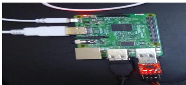
Figure 2. Raspberry PI-3 Model B.
